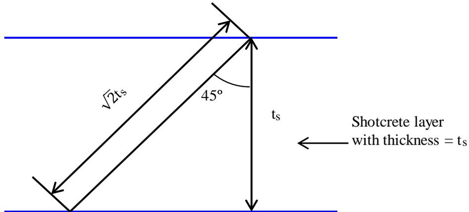
Figure 10. Thickness of shotcrete along the expected shear plane.
