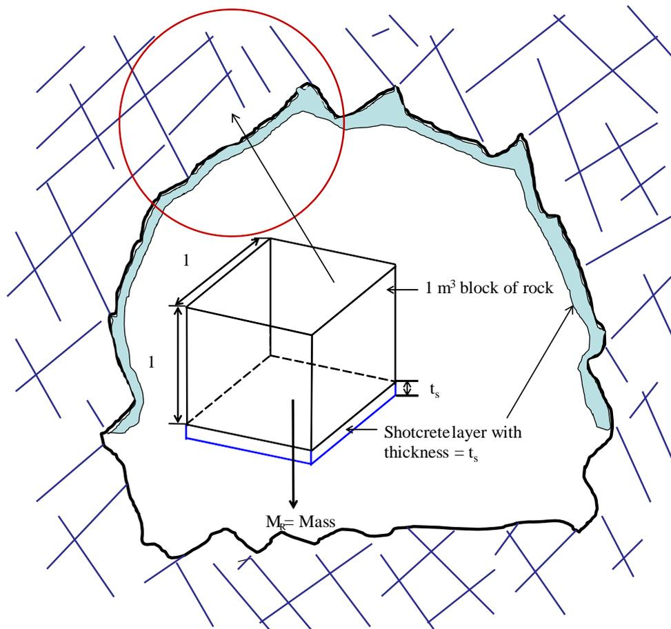
Figure 9. A 1 m<sup>3</sup> block of rock interacting with a shotcrete layer of thickness ( $t_s$ ).
