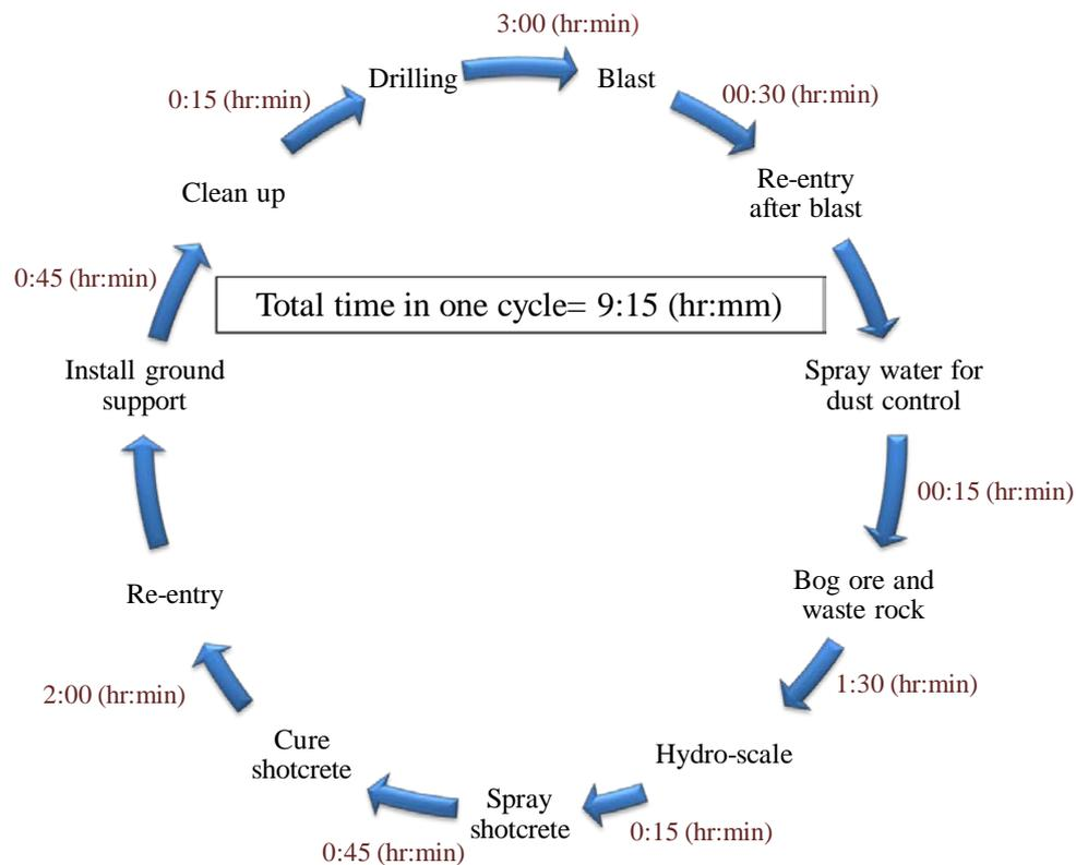
Figure 1. Underground mining process with ICS, (Width = 5.3m, Height = 5.5m, Advance = 3m. shotcrete thickness = 50mm) (Modified after O’Shea, 2005).
