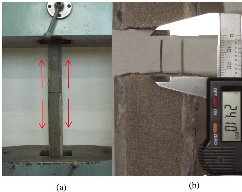
Figure 7. (a) The fibre pull-out test using an Avery Universal Testing Machine, and, (b) the fibre after pull-out.
