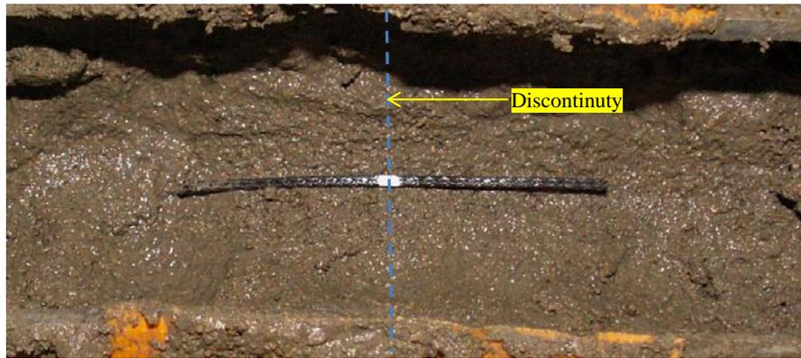
Figure 6. Installation of synthetic fibre across a simulated discontinuity for pull-out testing.
