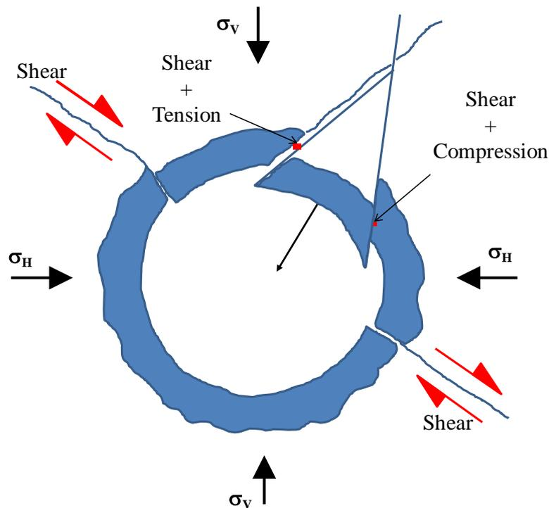
Figure 3. Shotcrete layer undergoing shear, a combination of shear and compression, and a combination of shear and tension (Windsor, 1999).
