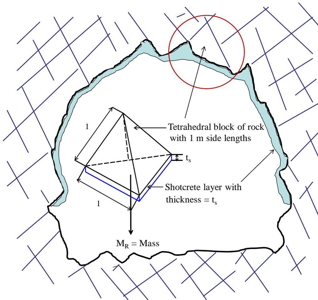
Figure 11. An equilateral tetrahedral block of rock with shotcrete layer with thickness ( $t_s$ ).
