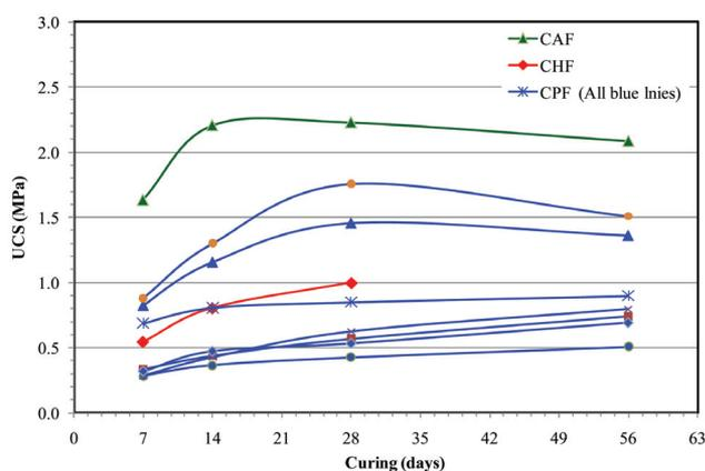
Figure 21—UCS development of CPF, CHF and CAF sample mix with 4% cement
