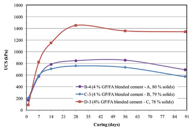
Figure 12—Average UCS development with time (GP/FA blended cement A, B and C)
