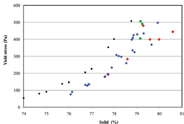
Figure 7—Typical correlation between solids density and yield stress of different CPF mixes
