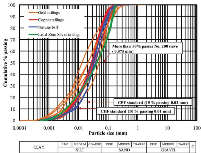
Figure 2—Typical particle size distribution curves of tailings and natural tuff
