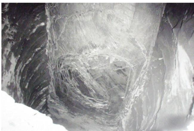
Figure 1—Secondary stope extraction using cemented hydraulic fill
