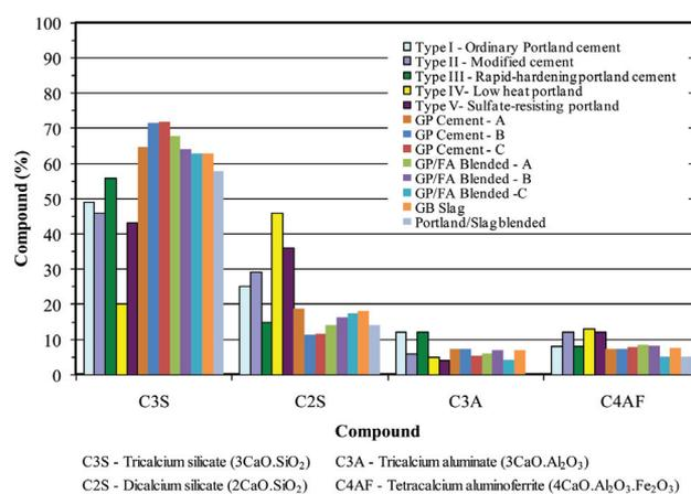
**Figure 6—Composition of the main compounds for a number of cement types**
