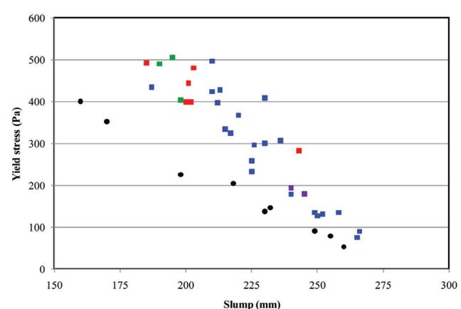
Figure 8—Typical correlation between yield stress and slump of different CPF mixes
