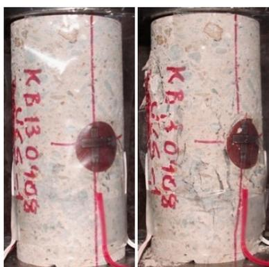
Figure 3. Shotcrete sample before and after UCS test.
