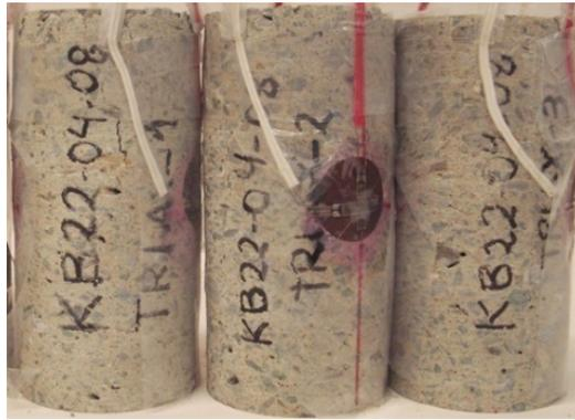
Figure 10. Samples after triaxial test.
