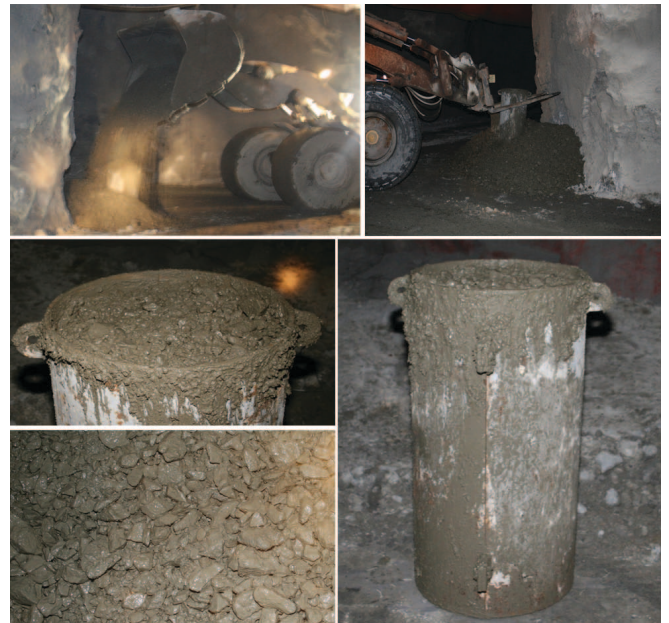
FIG 23 – Mixing and filling cemented rock fill samples for quality assurance/quality control test at Cosmos nickel mine.
