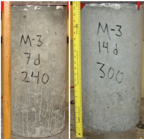
FIG 9 – Seven- and 14-day samples with high fines content.
