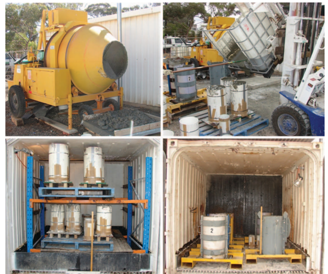
FIG 2 – Concrete mixer, sample casting and curing in the Western Australian School of Mines curing chamber.
