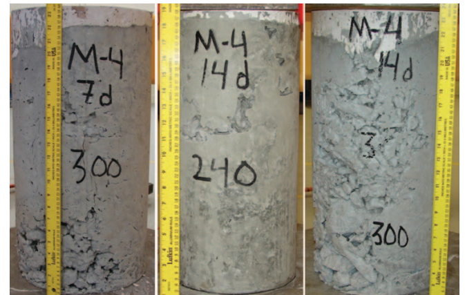
FIG 13 – Very high strength samples due to them being very well compacted and having low porosity and a high fines content.
