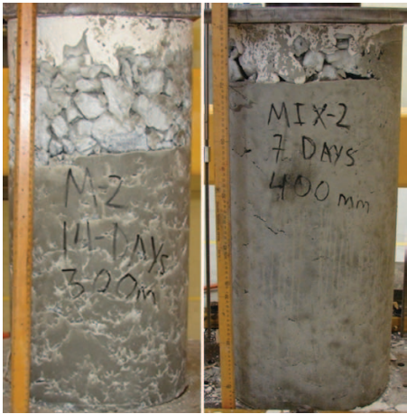
FIG 8 – Segregation in mix 2, thereby resulting in low strength.
