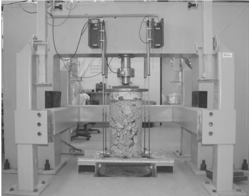
Figure 3. WASM static test machine set up for large scale UCS test.
