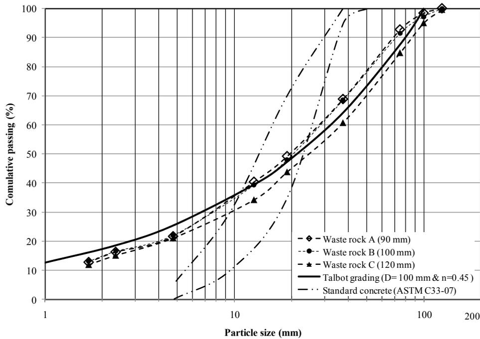
Figure 1. Particle size distribution curves of waste rock from Cosmos nickel mine.
