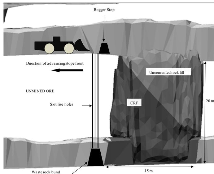
Figure 5. Schematic of cemented and uncemented rock filled stope (After, Van Der Merwe, 2009).
