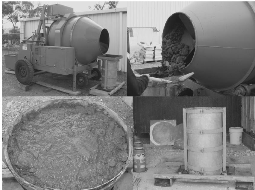
Figure 2. Concrete mixer, CRF mixing, sample casting and curing.
