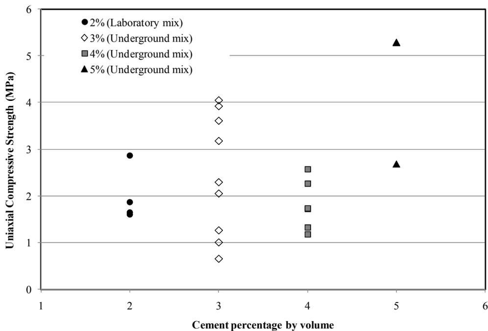
Figure 6. Comparison of UCS for CRF mixed in laboratory and underground.
