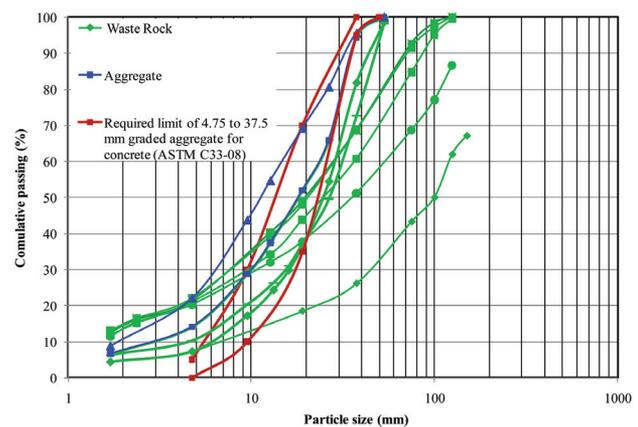
Figure 4—Typical particle size distribution curves of waste rock
