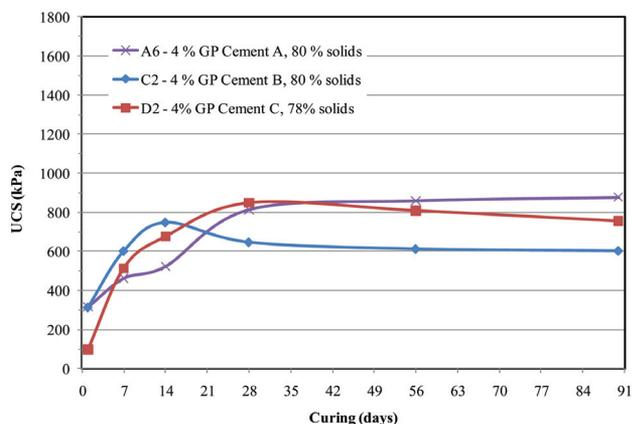
Figure 11—Average UCS development with time (GP cement A, B and C)
