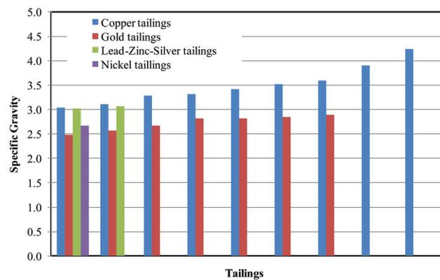
Figure 5—Typical specific gravity of tailings
