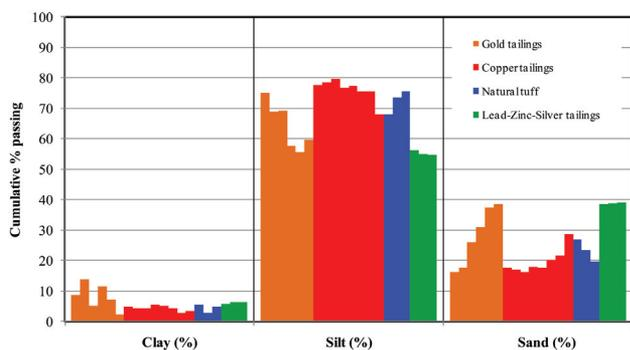
Figure 3—Typical particle size of tailings and natural tuff
