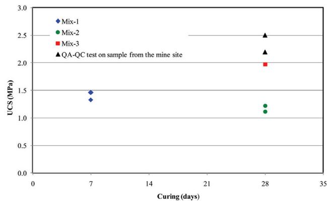
Figure 20—UCS development of CRF large-scale sample
