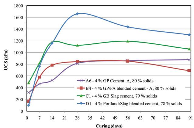
Figure 13—Average UCS development with time (GP A, GP/FA blended A, GB slag and Portland/slag blended cement)
