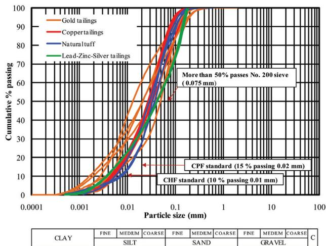
Figure 2—Typical particle size distribution curves of tailings and natural tuff
