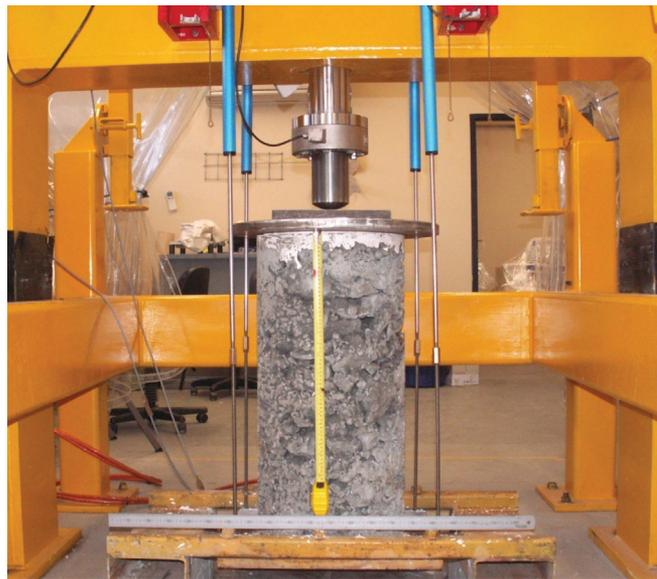
Figure 19—CRF sample (400 × 800) mm set up for UCS test
